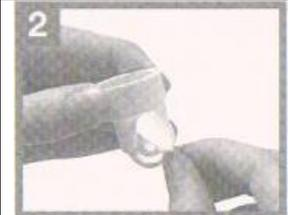
A close-up photograph showing a person's hands applying a small, white, circular membrane to a yellow piston inside the pump's head. The piston is partially inserted into a slot.       | 請將白色薄膜覆蓋在黃色活塞上，注意黃色活塞上是否有乳垢及毀損，乳垢及毀損會影響吸力。清洗時，白色薄膜需拆下清洗，用海綿或軟布清洗，請勿使用毛刷以免影響吸力。 |
